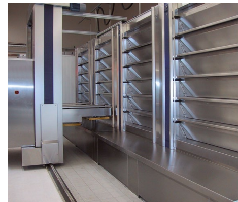
Example of a customised system: 4 HEIN ELECTRO deck oven with six decks each and the fully automatic HEIN SPIDER loading and unloading system.
